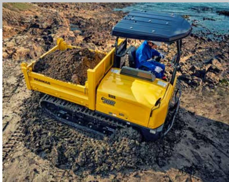
Spin turn by reverse turning both crawlers
