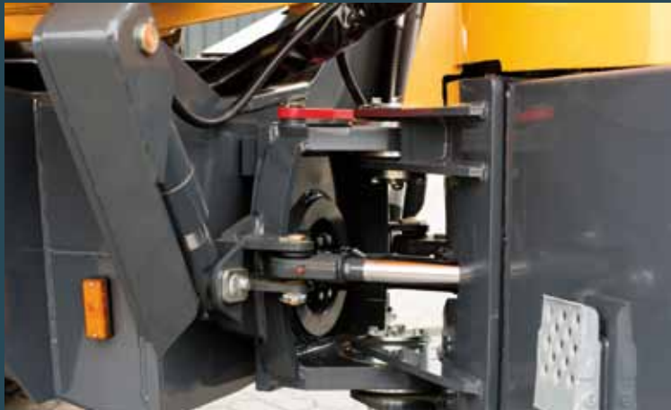
Articulated swivel joint with stabilisation cylinder.
