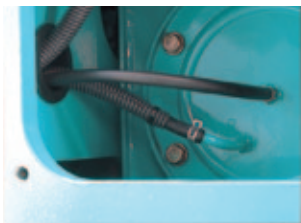
Fuel tank equipped with bottom flange and large drain valve
