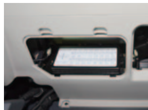
Easy-access fuse box. More finely differentiated fuses make it easier to locate malfunctions.
